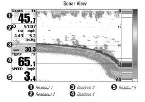
**Chart Views:** Readouts 1, 3, and 4 can be customized. Readout 2 (Heading) and Readout 5 (Speed) are fixed and cannot be customized.
