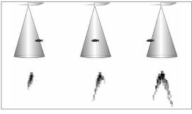
Transducer Cone and Fish Arches
