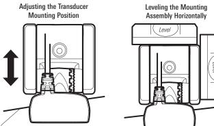
Seam aligned with boat hull
