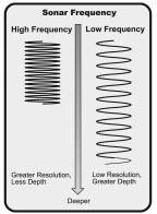
The sound pulses are transmitted at various frequencies depending on the application. Very high frequencies (455 kHz) are used for greatest definition, but the operating depth is limited. High frequencies (200 kHz) are commonly used on consumer sonar and provide a good balance between depth performance and resolution. Low frequencies (83 kHz) are typically used to achieve greater depth capability.
