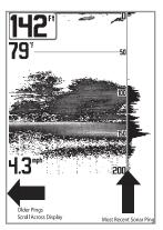
When all the echoes are viewed side by side, an easy to interpret "graph" of the bottom, fish and structure appears.
