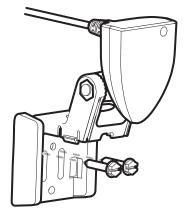
**NOTE:** Make sure that the mounting screws are snug, but do not fully tighten the mounting screws at this time to allow the transducer assembly to slide for adjustment ourposes.
