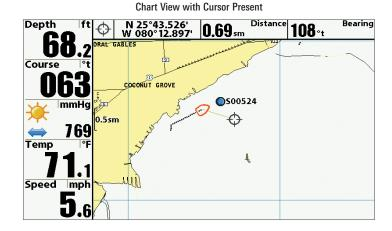
**Zooming:** Press the Plus (+) key to Zoom In and the Minus (-) key to Zoom Out to see the cartography at different magnification levels. The zoom level is indicated on the left side of the display. If you zoom in beyond the available chart data, the display will go into Overzoom mode whereby the last available chart data is amplified to reflect the level selected. If you zoom in so far that no cartography is available, a lat/long grid will be drawn instead.
