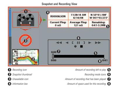
**NOTE:** For snapshots and recordings, the indicator bar has several states: during recording, the amount of space remaining on the MMC/SD card is indicated on the status bar. During playback, the amount of time/memory remaining to play is indicated on the status bar. When a snapshot thumbnail is highlighted, the amount of room remaining on the MMC/SD card is indicated.
