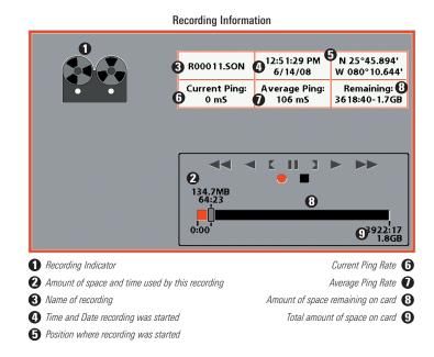
**NOTE:** Sonar chart speed is increased during Fast Forward and reversed during Rewind. This may reduce the quality of the sonar image, since at higher speeds, not every sonar return can be processed and displayed.
