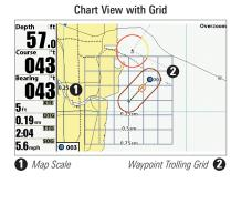
Add a Waypoint Target: From the Waypoints submenu, select Target, and press the RIGHT Cursor key to display the saved waypoints list. Select a waypoint and press the RIGHT Cursor key.
