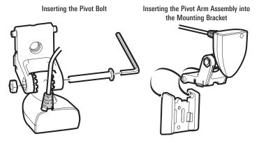
Put the pivot bolt through the assembly to hold it in position and loosely install the nut, but do NOT tighten the nut at this time. Insert the pivot arm assembly into the mounting bracket. Do NOT snap the assembly closed, as you will need to access the mounting bracket in the next step.
