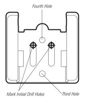
To lock down the transducer, trace the position of the mounting bracket. Force the pivot to the Up position to gain access to the mounting screws, then re-align the mounting bracket against the transom of the boat to match the traced silhouette. Check the bracket position with the level again to make sure it is still level, then mark the fourth mounting hole using a pencil or marker. Unscrew and remove the mounting screws and the transducer assembly and set aside.
