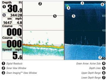
Down Imaging<sup>™</sup>/Sonar Combo View
