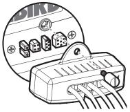
10. While holding cables in place in the cable collector insert, thread the cables through the slot in the bottom of the cable collector cover, line up the cable collector insert and cover, then slide the cover into place on the insert.
