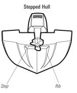
The best way to locate turbulence-free water is to view the transom while the boat is moving. This method is recommended if maximum high-speed operation is a high priority. If this is not possible, select a location on the transom where the hull forward of this location is smooth, flat and free of protrusions or ribs.
