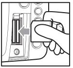
Inserting an MMC/SD into the Card Slot
