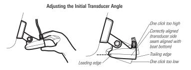
7. Adjust the transducer assembly vertically, until the seam on the leading edge of the transducer (the edge closest to the transom of the boat) is level and just slightly below the hull.
