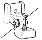
3. Re-position the transducer assembly against the transom of the boat, then hand install the first three screws (two on the outside edges and one in the 3rd mounting hole). Make sure that the transducer location and the pivot angle have not changed, then fully tighten all three mounting screws. Hand tighten only!
