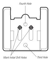
Continue to hold the bracket on the transom of the boat, and use a pencil or marker to mark where to drill the two mounting holes. Mark the drill holes near the top of each slot, making sure that your mark is centered in the slot.
