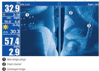
Submerged Bridge, Creek Channel, and New Bridge Piling
