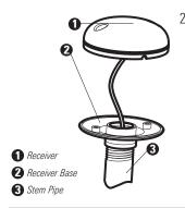
2. Screw on the receiver base to the stem first, making sure that the stem pipe does not protrude from the receiver base. This adds protection to the cable when pulling it through the pipe stem. In addition to this, de-burr the pipe edges to reduce cable abrasion.
