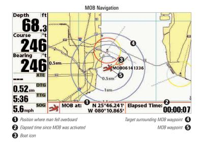
It is not possible to re-activate MOB or modify the current route without first canceling MOB navigation. The Off Course trigger is also disabled and the Off Course Alarm circle is not drawn. Any press of the GOTO key, or selection of a GOTO menu option, will cause an error beep and a short message will be displayed that will disappear after 2 seconds.
