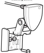
8. Re-position the transducer assembly against the transom of the boat, then hand-install all three screws. Make sure that the transducer location and the pivot angle have not changed, then fully tighten all three mounting screws. Snap the pivot back down. If you have performed the preceding procedures correctly, the transducer should be level and at the right height for optimal operation.
