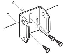
5. Align the metal mounting bracket with the mounting holes. The center slot should be above the two outer slots. (This bracket and all other hardware supplied is top quality stainless steel for maximum strength and corrosion protection.) Insert the three #10 - 1" long screws into the drilled holes, but do not completely tighten.
