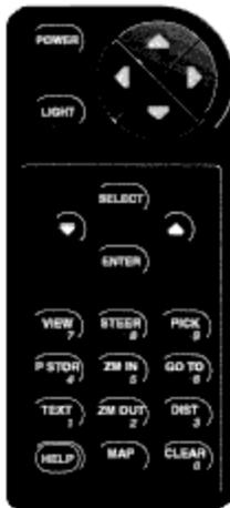
**LIGHT:** Multiple pushes of this key will adjust the level of light. The light is set at intensity level 2 when the unit is turned on. There are four intensity positions plus "OFF".
