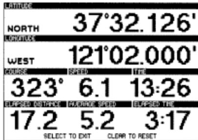
The DATALOG menu displays your latitude, longitude, course, speed, time, elapsed distance, average speed and elapsed time.
