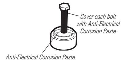
Figure 5. Securing the Antenna with Bolts and Washers in Four Locations
