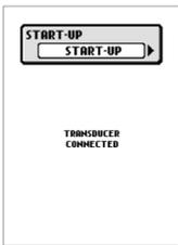
When the RF15 powers on, the Start-Up menu temporarily appears. From this menu, use the arrow keys to select either Start-Up, Simulator, or Setup. If you do nothing, the unit will default to normal on the water use.
