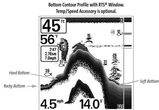
The sonar returns from the bottom, structure and fish can be represented as either **WhiteLine®** or **Structure ID®**. See *Sonar Menu Tab: Bottom View* for details on how to set the bottom view.
