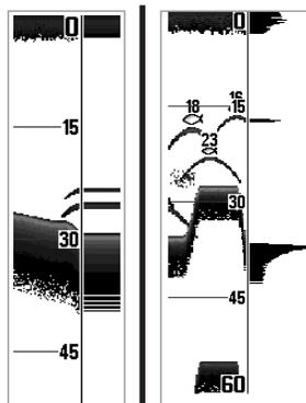
The **Wide RTS® Window** indicates the sonar intensity through the use of a bar graph. The length of the plotted return provides an indication of whether the return is weak or strong. The depth of the sonar return is indicated by the vertical placement of the return on the display depth scale.
