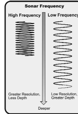
The sound pulses are transmitted at various frequencies depending on the application. Very high frequencies (455 kHz) are used for greatest definition but the operating depth is limited. High frequencies (200 kHz) are commonly used on consumer sonar and provide a good balance between depth performance and resolution. Low frequencies (83 kHz) are typically used to achieve greater depth capability.
