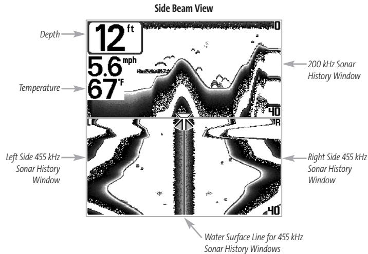
The sonar information from the side-looking beams reveals bottom contour, structure and fish similar to the down-looking beam, but the area covered is to the left and right of the area shown in the down-looking portion, so you actually see more of the bottom. The distance covered by the right and left 90° beams is based on the depth setting for the down-looking beam, up to a maximum of 160 feet.
