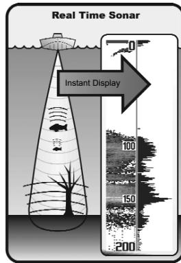
SONAR is an acronym for **SO**und and **NA**avigation **R**anging. Sonar utilizes precision sound pulses or "pings" which are emitted into the water in a teardrop-shaped beam.
