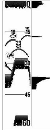
The **Wide RTS™ Window** indicates the sonar intensity through the use of a bar graph. The length of the plotted return provides an indication of whether the return is weak or strong. The depth of the sonar return is indicated by the vertical placement of the return on the display depth scale. The Wide RTS™ Window does not make use of grayscale.
