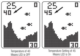
2. To change the setting to 45°F (7°C) (blinking light ON) touch and release the wet switch contacts once more. Wait two seconds and then confirm that the temperature reading on the Control Head has changed to 45°F (7°C). Single touches will toggle the setting between 40°F (4°C) and 45°F (7°C).
