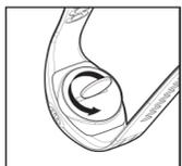
Make sure that the O-ring in the battery compartment is present, positioned correctly in the grooves, and free of debris before re-installing the battery door.
