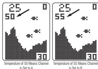
2. To change the setting to 55°F (12°C) (channel set to B) touch and release the wet switch contacts once more. Wait two seconds and then confirm that the temperature reading on the Control Head has changed to 55°F (12°C). Single touches will toggle the setting between 50°F (9°C) and 55°F (12°C).
