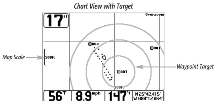
**Add or Remove a Trolling Grid:** From the Waypoints submenu, select Grid and press the RIGHT Cursor key to display a list of waypoints. Select the waypoint to which you want to add the grid. The trolling grid will appear on all of the navigation views, and can be used as a guide when trolling around a waypoint. The grid can be rotated to any desired heading using Grid Rotation from the Navigation Main menu. To remove the trolling grid, choose Remove Grid from the Navigation X-Press™ menu.
