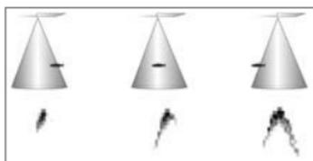
*Transducer Cone and Fish Arches*
