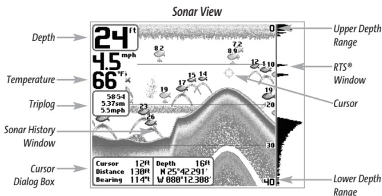
**NOTE:** If the Depth number is flashing, it means that the unit is having trouble locating the bottom. This usually happens if the water is too deep, the transducer is out of the water, the boat is moving too fast, or for any other reason that the unit can't accurately receive continuous data.
