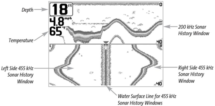
The sonar information from the side-looking beams reveals bottom contour, structure and fish similar to the down-looking beam, but the area covered is to the left and right of the area shown in the down-looking portion, so you actually see more of the bottom. The distance covered by the right and left 90° beams is based on the depth setting for the down-looking beam, up to a maximum of 160 feet.
