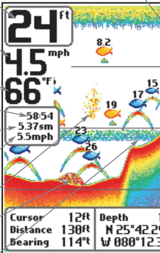
**Cursor Dialog Box** - indicates cursor depth on the display. In addition, the Latitude and Longitude of the cursor position and the bearing to the cursor position. A waypoint
