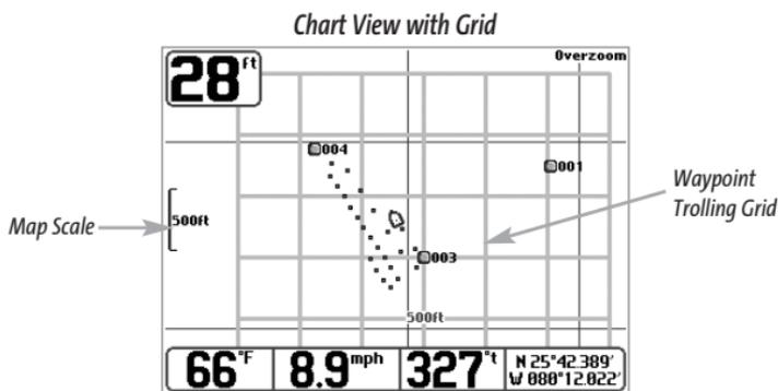
**NOTE:** Only one waypoint can have either a target or a grid at one time. If you apply a target or a grid to a new waypoint, the original waypoint will lose its target or grid.
